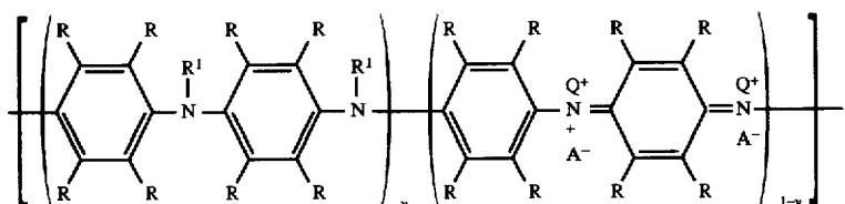
50 The emeraldine salt is the highly conducting form. The conductivity of the polyaniline can range from  $10^{-10} \text{ ohm}^{-1} \text{ cm}^{-1}$  (characteristic of the base and non-doped form) to about  $10^3 \text{ ohm}^{-1} \text{ cm}^{-1}$  upon full doping.
