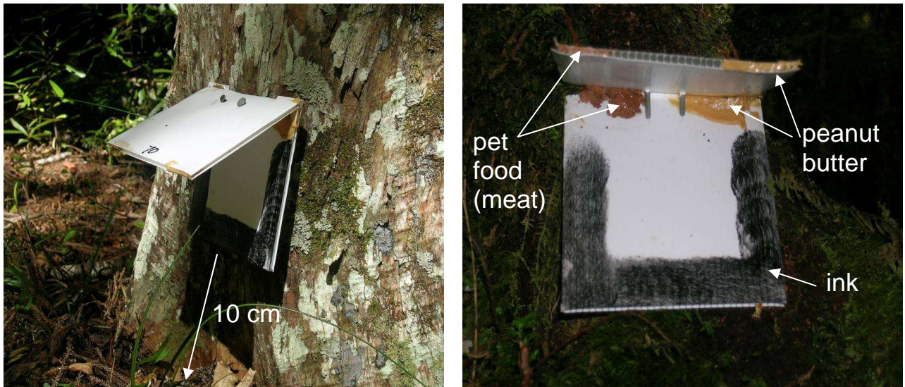
Figure 3. ChewTrack Card design, showing (a) side view, and (b) the location of tracking ink and bait (peanut butter for possums and rodents, meat paste for rodents, stoats and other carnivores).
