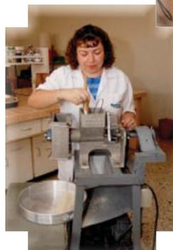
The low cost Omega VI Grinder produced by the NGO, Compatible Technologies International, Minneapolis, MN, USA is designed for family use in rural areas of developing countries. The grinder produces excellent sorghum flour for baking.
