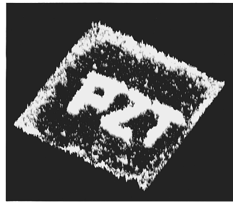
FIG. 3. Three-dimensional image of a polarization-induced "PZT" pattern written in the PZT-0.8 film. A dark square of 4 \times 4 \mu\text{m}^2 was produced by scanning the SFM tip while applying a positive 20 V pulse. The "PZT" film character seen in the figure, produced by moving the SFM tip while applying a negative 10 V signal, exhibit opposite piezoelectric coefficients and opposite polarities (positive and negative, respectively). The gray region corresponds to a nonpolarized area, which does not show piezoelectric response. The scanning area is 5 \times 5 \mu\text{m}^2 .
