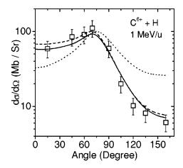
FIG. 6. The energy integrated angular distributions  $d\sigma/d\Omega$  for 12 MeV C<sup>6+</sup> + H. The data are compared to the *B*1, CDW-EIS, and the CDW calculations using the different lines described in Fig. 2.
