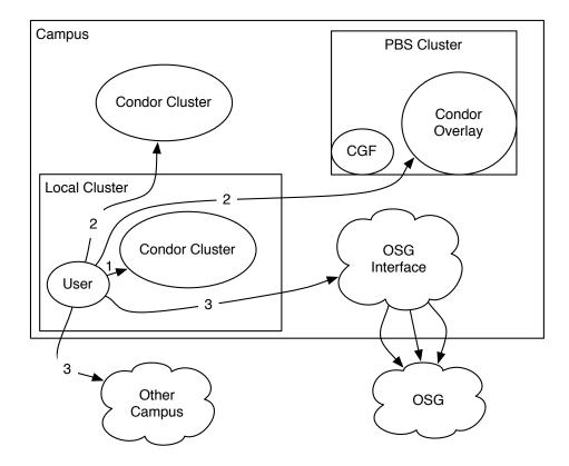
Figure 4.6: The Full Campus Grid Architecture
