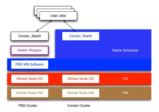
Figure 4.4: Layered Diagram of the Worker Node
