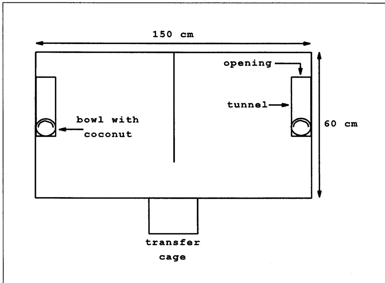
**FIGURE 1.** Schematic of stainless steel arena used to evaluate the repellency of mongoose (*Herpestes auropunctatus*) feces and urine to captive wild rats (*Rattus rattus* and *R. exulans*). The walls and incomplete partition were 120 cm tall. Rats had free access to two tunnels that each contained a bowl with a chunk of coconut. During treatment trials, one of the bowls was treated with water, mongoose feces, mongoose urine, or butyric acid.
