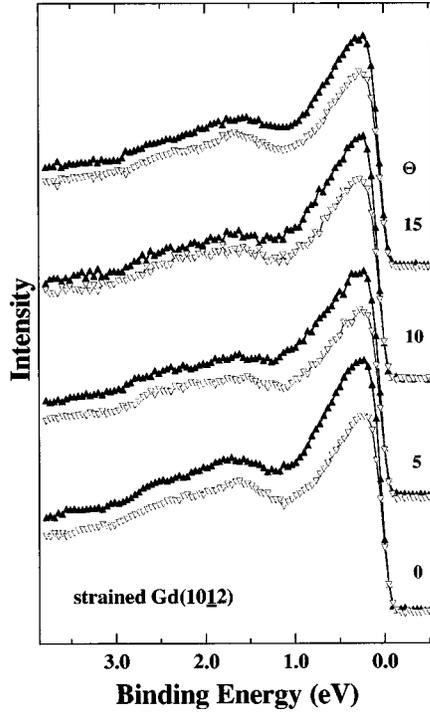
FIG. 8. Emission angle-dependent spin-polarized photoemission spectra of a 4-ML gadolinium film on Mo(112) at 145 K. These spectra of the “strained Gd(10 $\bar{1}2$ )” thin film exhibit little bulk band exchange splitting, the features at higher binding energies (see text).
