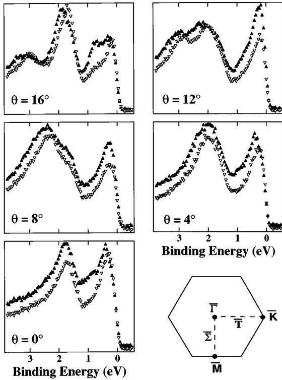
FIG. 4. Spin-polarized emission angle-dependent valence-band photoemission spectra for various points along the  $\bar{\Gamma}\bar{\Sigma}\bar{M}$  high-symmetry line. The spectra were acquired for a 40-ML-thick strained Gd film at approximately 145 K. Spin-majority and spin-minority components are indicated by ( $\blacktriangle$ ) and ( $\nabla$ ), respectively. The bottom right panel displays the hexagonal surface Brillouin zone of strained Gd.
