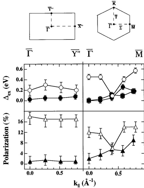
FIG. 6. The exchange splitting (top) and spin asymmetry *above* background (bottom) of the surface (open symbols) and bulk (filled symbols) spin subbands as a function of wave vector. Data are shown for a strained 4-ML-thick ( $10\bar{1}2$ ) thin film (left) and a 40-ML-thick (right) strained (0001) Gd film grown on Mo(112). The data points have been extracted from spin-polarized photoemission spectra at 145 K. The Brillouin-zone symmetry points are indicated at the top.
