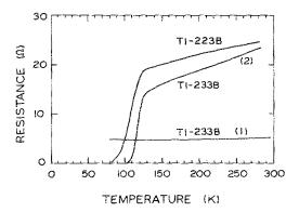
FIG. 2. Film Tl-223B was processed at too high a temperature (920 °C) and exhibits a substantially lower zero-resistance temperature than film Tl-223A. Curve (1) for film Tl-233B resulted when the film was processed at too low a temperature and for too short a time. Curve (2) shows R vs T for the same film after a second thermal cycle under the appropriate conditions.
