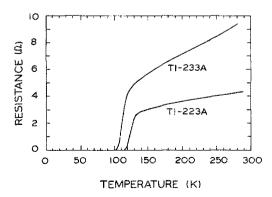
FIG. 1. Temperature dependences of resistance for a Tl<sub>2</sub>O<sub>3</sub> vapor processed Ba<sub>2</sub>Ca<sub>3</sub>Cu<sub>3</sub>O<sub>8</sub> thin film (T1-223A) and a Tl<sub>2</sub>O<sub>3</sub> vapor-processed Ba<sub>2</sub>Ca<sub>2</sub>Cu<sub>3</sub>O<sub>7</sub> thin film (T1-233A).
