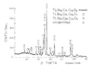
FIG. 3. X-ray diffraction scan of film Tl-223A. The 2212 phase peaks are indexed, while the 1212 and 1223 phase peaks are also identified. All these peaks indicate *c*-axis orientation. There are also two unidentified peaks in the scan.
