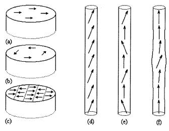
FIG. 1. Spin-wave modes in nanowires: (a) and (d) coherent mode, (b) curling mode, (c) bulk mode with  $k_{\perp} > 1/R$ , (e) mode with  $k_{\parallel} > 0$ , and (f) localized nucleation mode. The bulk modes are essentially superpositions of plane waves. Since the diameter of typical nanowires is much larger than the interatomic distance, there are many excited perpendicular modes, and the finite-temperature magnetization  $M_s(T)$  is reminiscent of bulk magnets.
