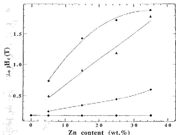
FIG. 1. Coercivity  $H_c$  vs Zn content for different heat treatments conditions: before heat treatment;  $\blacklozenge$ —390 °C for 100 min;  $\blacktriangle$ —390 °C for 300 min;  $+$ —425 °C for 100 min,  $\bullet$ —mixed powder.
