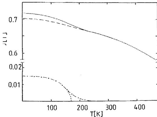
FIG. 6. Thermomagnetic phase analysis for the magnet of Fig. 5: —, experimental polarization-versus-temperature curve measured on the major demagnetization curve at an applied field of 1 T; ---,  $T^{3/2}$  fit for the low-temperature behavior of the magnetic main phase; - · - ·, resulting  $J$ -vs- $T$  curve for an additional ferromagnetic phase; ··· extrapolation to zero-field condition.
