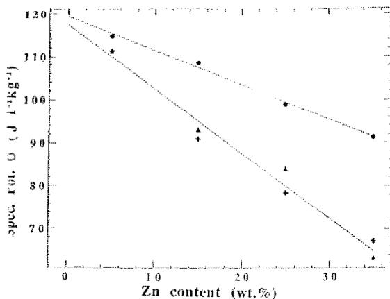
FIG. 3. Specific polarization  $\sigma$ , measured at an external field of 4 T, as a function of Zn content for different heat treatments conditions: ●—before heat treatment; ▲—390 °C for 300 min; +—425 °C for 100 min.
