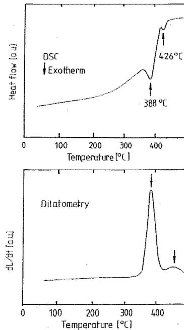
FIG. 4. Differential scanning calorimetry (DSC) curve (heating rate 20 K/min) and dilatometry curve (heating rate 10 K/min) for a sample made from a mixture of  $\text{Sm}_2\text{Fe}_{17}\text{N}_x$  with 15 wt % Zn.
