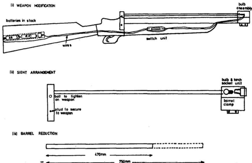
Figure 8. Modification of standard shotgun for night hunting.
