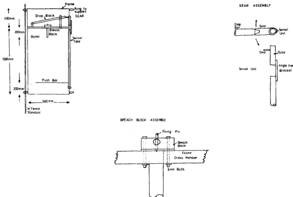
Figure 3. The frame design for a trap gun.
