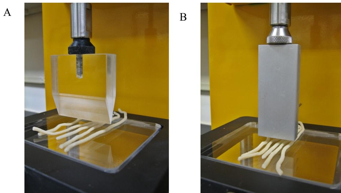
Figure 3A. TPA testing with wedged TA-PFS probe
