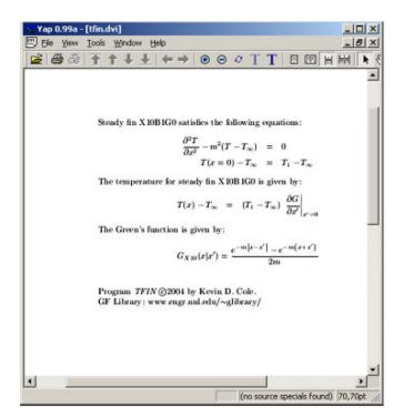
**Figure 2.** Output of program TFIN for the temperature in a fin, case X10B1G0, showing an expression for temperature, along with the associated differential equation, heating conditions, and Green's function.
