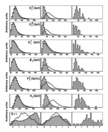
FIG. 3. Monte Carlo distributions for the seven variables used in the ANN. In the left plots, the open (shaded) histograms correspond to the  $W^*$  (Wg) channel. Similarly, in the middle-column plots open (shaded) histograms correspond to  $t\bar{t}$  (W+ jets). All Monte Carlo distributions are normalized to unit area for comparison. The histograms in the right column correspond to the run I data events.
