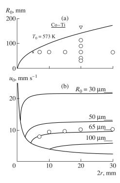
**Fig. 4.** Nanodiabatic combustion behavior for the Co–Ti system with stoichiometric mixture at  $T_0 = 573$  K: (a) Range of flammability as a function of 2r and  $R_0$ , data are from Itin et al.; ( $\bigcirc$ ) designates the steady propagation, ( $\square$ ) the flame extinction during the propagation, and ( $\times$ ) the non-ignition. (b) Burning velocity  $u_0$  as a function of 2r, with  $R_0$  taken as a parameter, data points are experimental in the literature.
