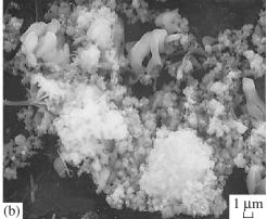
**Fig. 7.** SHS produced  $\beta$ -Si<sub>3</sub>N<sub>4</sub> (a) and  $\alpha$ -Si<sub>3</sub>N<sub>4</sub> (b).
