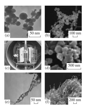
**Fig. 5.** (a), (b) TEM images of Al and Ni nanoreactants, (c) reaction chamber, (d) SEM image of nanosized nickel aluminide–alumina composite prepared by simultaneous combustion synthesis and densification, (e), (f) SEM images of single-walled carbon nanotubes reinforced nickel aluminide–alumina nanocomposites.
