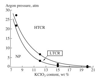
**Fig. 6.** Combustion propagation diagram in Si–C–KClO<sub>3</sub> reacting system: NP means no propagation; LTCR stands for low temperature combustion regime; and HTCR, for high temperature combustion regime.
