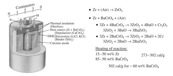
**Fig. 1.** Use of zirconium in thermal batteries [16].
