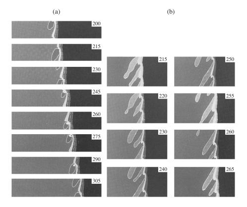
Fig. 3. Two-dimensional modeling: (a) single head spinning wave and (b) multiple head spinning waves [64].
