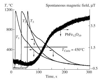
Fig. 9. Three temporal combustion temperatures in the top  $(T_1)$ , middle  $(T_2)$ , and bottom  $(T_3)$  of the sample and the spontaneous magnetic field measured near the one side of the sample during the combustion synthesis of ferrite. The distance between surface and sensor was 10 mm [226].
