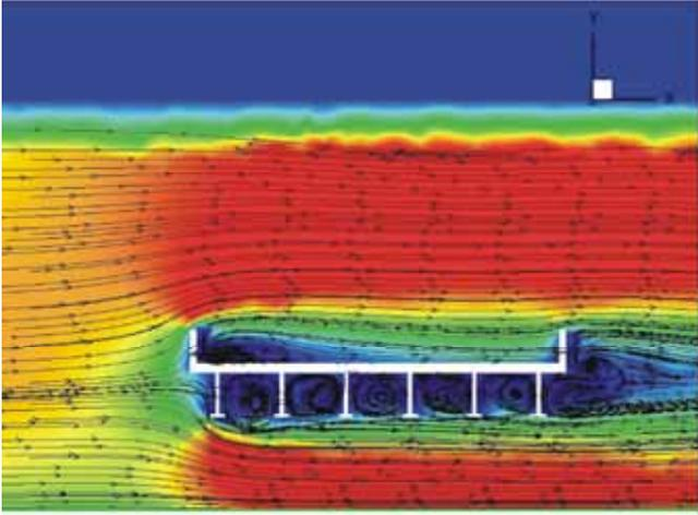
**Figure 22. Image. Velocity profile from the Fluent<sup>®</sup> k-ε CFD model for the six-girder bridge.**
