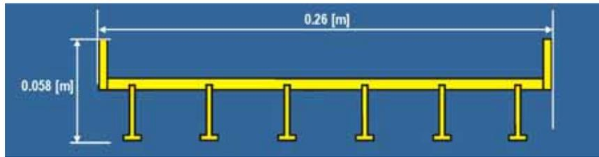
**Figure 8. Diagram. Dimensions of the six-girder bridge deck.**
