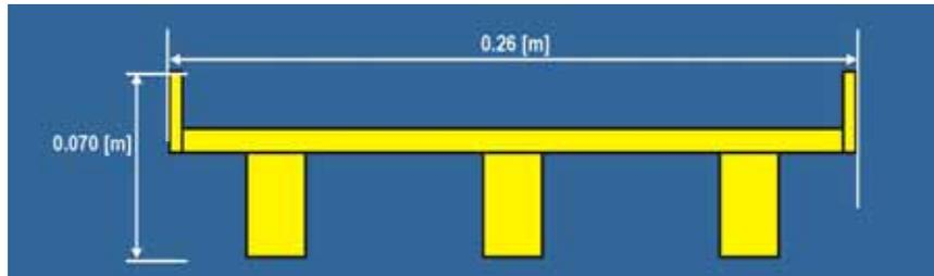
**Figure 9. Diagram. Dimensions of the three-girder bridge deck.**
