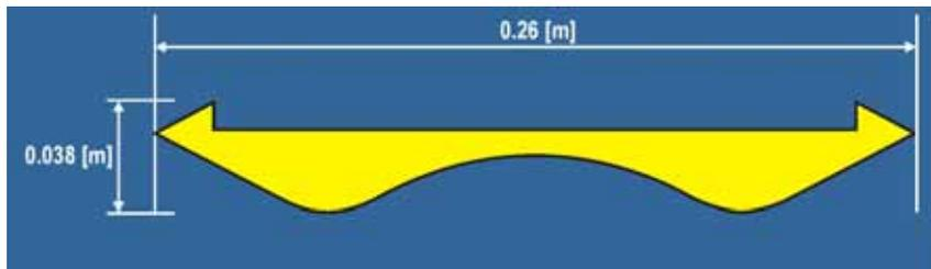
**Figure 10. Diagram. Dimensions of the streamlined bridge deck.**
