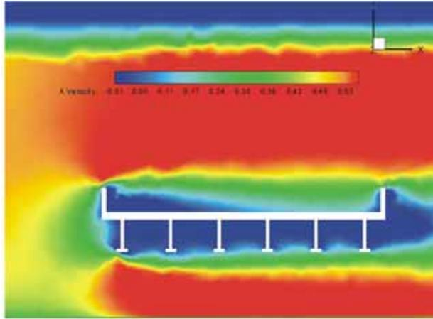
**Figure 20. Image. Velocity profile from the 3-D Fluent<sup>®</sup> model.**
