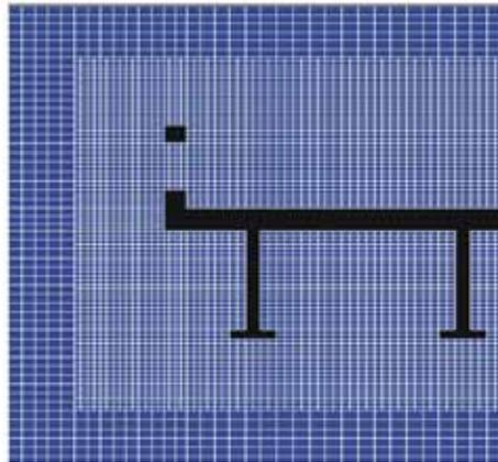
**Figure 17. Diagram. Partially refined meshes for STAR-CD<sup>®</sup> simulation.**
