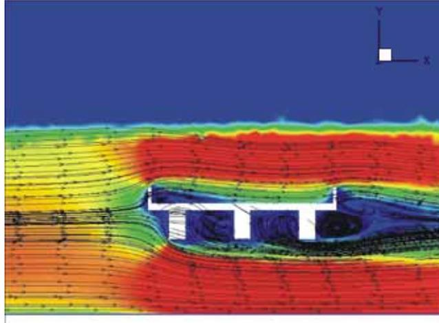
Figure 24. Image. Velocity profile from the Fluent<sup>®</sup> k-ε CFD model for the three-girder bridge.
