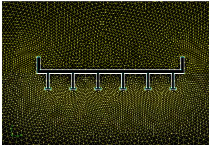
**Figure 21. Diagram. Fluent<sup>®</sup> unstructured mesh in the vicinity of the bridge.**
