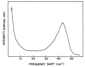
FIG. 3. Raman spectrum of the unstable mode at  $128\,^{\circ}\mathrm{C}$  and 2.8 kbar.
