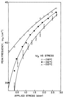
FIG. 2. Change in peak frequency with stress.
