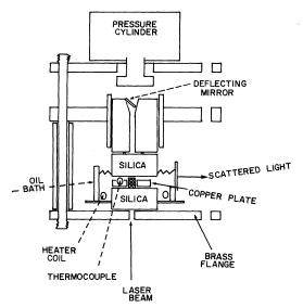
FIG. 1. Schematic diagram of uniaxial stress cell.
