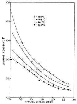
FIG. 4. Stress dependence of the damping constant  $\Gamma$ .
