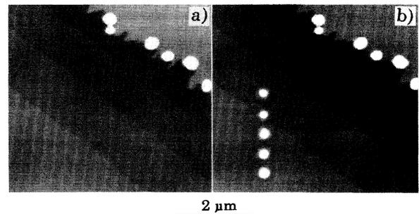
FIG. 2. AFM topography images before (a) and after (b) the application of local electric field by the AFM tip, resulting in the creation of an array of five circular domains. Diagonal grey bands are the monatomic lattice steps of about 0.8 nm height.
