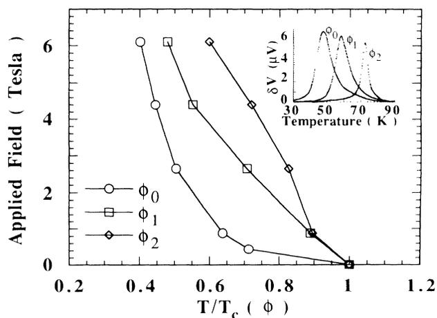
FIG. 4. Irreversibility line before ( $\phi_0$ ) and after irradiation at  $\phi_1=1 \times 10^{11}$  and  $\phi_2=3 \times 10^{11}$  ions/cm<sup>2</sup>. Inset: The quadrature ( $\chi''$ ) component of the pickup voltage at 4.4 T before and after irradiation.
