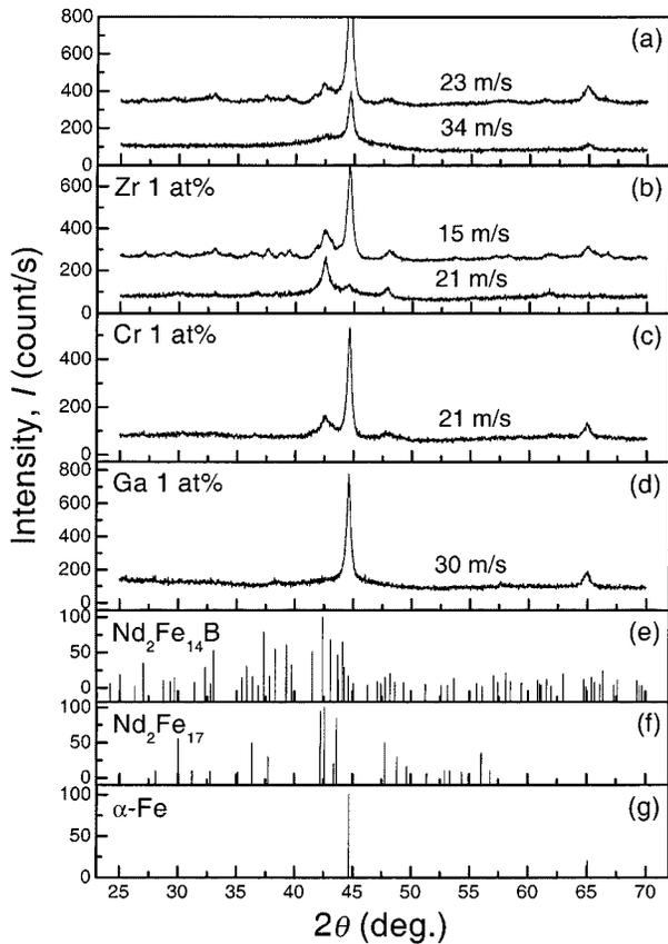
Fig. 1. XRD patterns of melt-spun (a)  $\text{Nd}_{10}\text{Fe}_{82}\text{B}_2\text{C}_6$ ; (b)  $\text{Nd}_{10}\text{Fe}_{81}\text{ZrB}_2\text{C}_6$ ; (c)  $\text{Nd}_{10}\text{Fe}_{81}\text{CrB}_2\text{C}_6$ ; (d)  $\text{Nd}_{10}\text{Fe}_{81}\text{GaB}_2\text{C}_6$  ribbons. The reference patterns of the  $\text{Nd}_2\text{Fe}_{14}\text{B}$ ,  $\text{Nd}_2\text{Fe}_{17}$ , and  $\alpha\text{-Fe}$  phases are shown in (e), (f), and (g), respectively.
