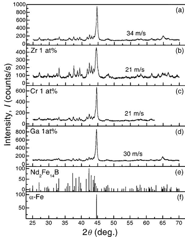
Fig. 2. XRD patterns of optimally melt-spun ribbons followed by optimal annealing: (a)  $\text{Nd}_{10}\text{Fe}_{82}\text{B}_2\text{C}_6$ ; (b)  $\text{Nd}_{10}\text{Fe}_{81}\text{ZrB}_2\text{C}_6$ ; (c)  $\text{Nd}_{10}\text{Fe}_{81}\text{CrB}_2\text{C}_6$ ; (d)  $\text{Nd}_{10}\text{Fe}_{81}\text{GaB}_2\text{C}_6$  ribbons. The reference patterns of the  $\text{Nd}_2\text{Fe}_{14}\text{B}$ , and  $\alpha\text{-Fe}$  phases are shown in (e), and (f), respectively.
