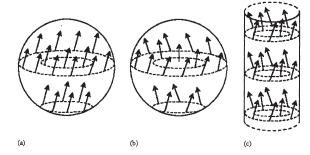
**Figure 10.** Nucleation modes in homogeneous magnets: (a) coherent rotation in a sphere, (b) curling in a sphere, and (c) curling in a cylinder. The arrows show the local magnetization  $M = M_x e_x + m$ , where  $e_x$  is parallel to the axis of revolution of the ellipsoid (cylinder).
