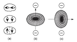
**Figure 5.** Physical origin of magnetic anisotropy: (a) compass-needle analogy of shape anisotropy and (b–c) magnetocrystalline anisotropy. In (b) and (c), the anisotropy energy is given by the electrostatic repulsion between the tripositive rare-earth ions and the negative crystal-field charges.
