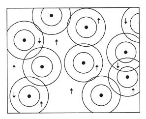
**Figure 2.** Carrier mediated exchange in dilute semiconductors (schematic). The mechanism is similar to RKKY interactions, but due to the essential involvement of donor or acceptor orbitals,  $J(r_i, r_i)$  can no longer be written as  $J(|r_i - r_i|)$ .
