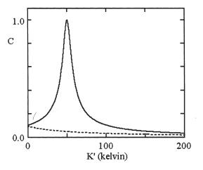
**Figure 21.** Entanglement as a function of the anisotropy K' of the second dot. The solid and dashed lines denote FM and AFM couplings, respectively. The parameters are  $S_o = S_o' = 1$ , N = 1000, N' = 1100, K = 50 K, and J = 0.005 K. For simplicity, H = 0 and H' = 0. The FM maximum is a resonance effect involving  $|01\rangle$  and  $|10\rangle$  states; there is no similar resonance in the AFM case.
