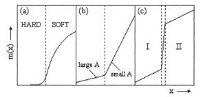
**Figure 19.** Boundary conditions and exchange: (a) hard-soft interface with common A, (b) interface between two ferromagnetic phases with different A, and (c) quasi-discontinuous magnetization due to strongly reduced exchange between grains I and II. Note that the perpendicular magnetization component m(x) can be interpreted as a magnetization angle.
