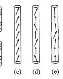
**Figure 13.** Spin-wave modes in nanowires: (a) is the coherent mode ( $k_{\perp} = 0$ ) and (b) is of the curling type. When  $k_{\perp} \gg 1/R$ , then the perpendicular spin waves are essentially superpositions of plane waves  $\exp(ik_{x}x)$  and  $\exp(ik_{y}y)$ . Since the diameter of typical nanowires is much larger than interatomic distance, there are many excited perpendicular modes, and the finite-temperature magnetization  $M_{\kappa}(T)$  is reminiscent of bulk magnets.
