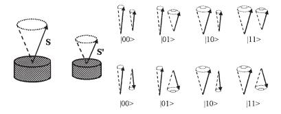
**Figure 20.** Quantum states of interacting nanodots. The dots (left) may be coupled ferromagnetic (top right) or antiferromagnetic (bottom right). The labels  $|0\rangle$  and  $|1\rangle$ , denote states where |m| = S and |m| = S - 1, respectively.
