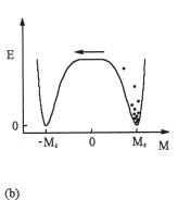
**Figure 15.** Dynamic hysteresis-loop effects: (a) magnetic viscosity and (b) sweep-rate dependence. The sweep-rate dependence amounts to a fluctuation-field [165] or sweep-rate correction to the static coercivity  $H_{co}$ .
