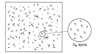
Figure 18. Cooperative spin blocks. When the size N of the particle becomes too big, then thermal activation leads to the formation of cooperative units of size N<sub>o</sub>.
