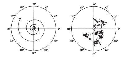
**Figure 12.** Magnetization dynamics of a nanoparticle: (a) damped precession and (b) random thermal motion. The curves are simulations for typical but not critical parameters, covering a time of order 0.1 ns. In both polar plots, the direction of the motion is from the white circles to the black circles.
