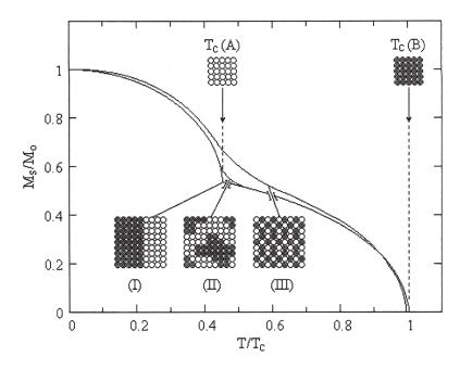
**Figure 4.** Spontaneous magnetization of inhomogeneous magnets: (I) macroscopic mixture, (II) nanostructure, and (III) alloy. In alloys and nanostructures, there is only one Curie temperature, although the  $M_s(T)$  curves of nanostructures exhibit a two-phase like inflection whose curvature may be difficult to resolve experimentally [36].
