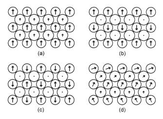
**Figure 1.** Spin structures (schematic): (a) ferromagnetism, (b–c) antiferromagnetism, and (d) noncollinear structure. The shown structure of the  $L1_0$  type; the small atoms (with the large magnetization arrows) the iron-series transition-metal atoms, as compared to the bigger 4d/4f atoms. Examples of  $L1_0$  magnets are CoPt and FePt.
