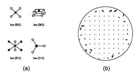
**Figure 6.** Surface anisotropy: (a) atomic origin and (b) realization in a nanoparticle. Lowest-order biaxial anisotropy is realized for bcc (011) but not for bcc (001) and bcc (111). The large surface-to-volume ratio of clusters leads to a comparatively strong diameter dependence of the intrinsic properties such as anisotropy [68] and magnetization.
