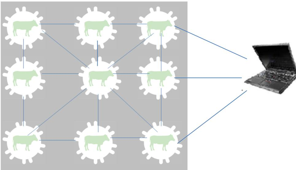
Figure 8. An example of packet transmission via multi-hops to base station
