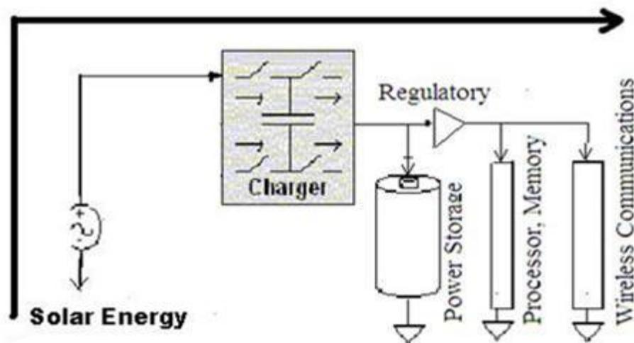
Figure 3. Electrical diagram of the energy-harvesting system
