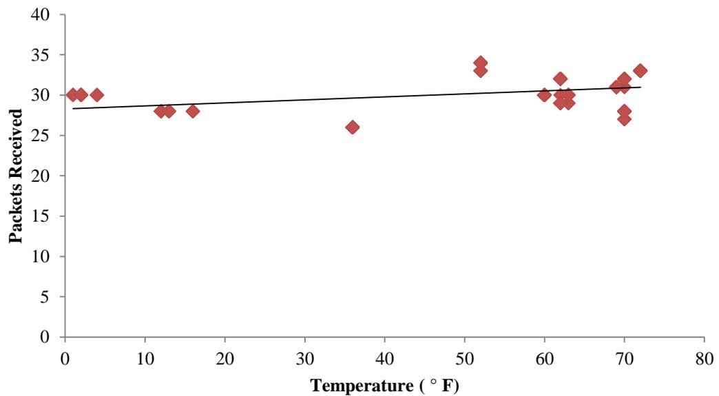
Figure 5. Effect of temperature on number of packets received.
