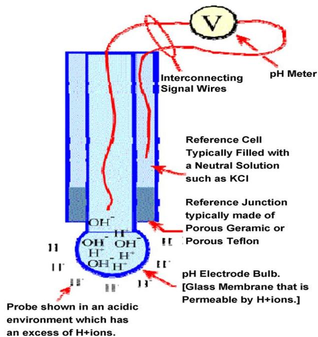
Figure 2. Diagram of pH sensor (Mottram et al., 2008)
