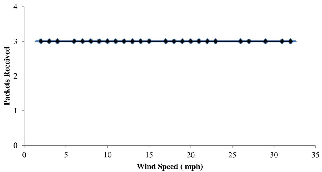
Figure 14. Effect of wind speed on number of packets received.
