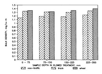
Fig. 3—Bulk density for the plow tillage treatment averaged over all water contents. Differences in bulk density between the rubber belt track and tire were significant at the 0.10 level only for the 225 to 300 mm depth.
