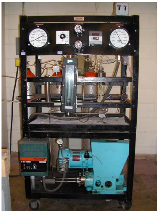
Fig. 1. Supercritical fluid processing unit.
