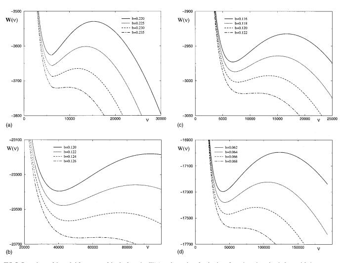
FIG. 7. Dependence of the scaled free energy of droplet formation  $W(\nu)$  on the number of molecules  $\nu$  for various given chemical potentials (or supersaturations). (a) and (c):  $\tilde{R}_n = 5d$ ; (b) and (d):  $\tilde{R}_n = 15d$ . (a) and (b):  $T^* = 0.7$ ; (c) and (d):  $T^* = 0.9$ . The thicker curves represent the region where the power-law approximation is applicable.
