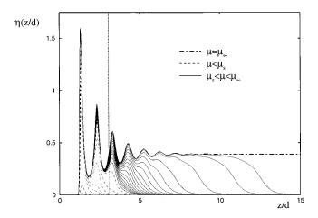
FIG. 2. The scaled density profile  $\eta(z/d) = \rho(z/d) \pi d^3/6$  of LJ fluid films near an LJ 9–3 smooth planar wall located at z=0, for various given chemical potential  $\mu$  at  $T^* = k_B T/\epsilon_{\rm LJ} = 0.9$ . The vertical dotted line represents the position  $z_0/d$ .
