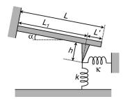
FIG. 1. Model for cantilever dynamics. The cantilever is a rectangular beam of length L that is clamped at one end. The cantilever is tilted at an angle  $\alpha$  with respect to the sample. The tip has length h and is located at a position  $L_1 = L - L'$  with respect to the clamped end. The tip is coupled to the sample by a vertical (normal) spring of stiffness k and a horizontal (tangential) spring of stiffness  $\kappa$ .
