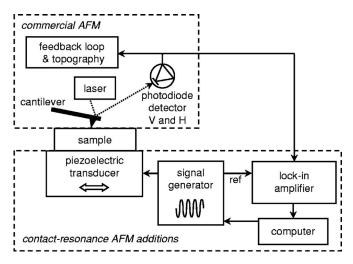
FIG. 3. Block diagram of experimental AFAM apparatus.
