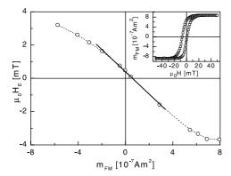
Fig. 1.  $H_{\rm e}$  vs.  $m_{\rm FM}$  dependence of the Fe<sub>0.6</sub>Zn<sub>0.4</sub>F<sub>2</sub>(110)/Fe14nm/Ag35nm heterostructure (circles). The data are obtained from the shifts of the magnetic hysteresis curves after cooling the system to  $T=10\,\rm K$  in an applied field which sets the target value  $m_{\rm FM}$ . The solid line shows a linear fit in accordance with proportionality (3). The inset shows a typical hysteresis after freezing in the saturated FM state.
