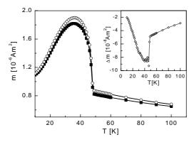
Fig. 2. m vs. T data measured with (squares) and without (circles) external shear stress  $\sigma_{xy} > 0$  applied along the [110] direction of the antiferromagnet. The inset exhibits the difference (diamonds) between both sets of data.
