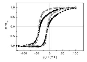
Fig. 3. Magnetic hysteresis after saturation of the FM layer at  $T=100\,\mathrm{K}$  and subsequent cooling in  $\mu_0H=5\,\mathrm{mT}$  to  $T=10\,\mathrm{K}$ . Circles indicate the hysteresis under natural shear stress. Squares exhibit the hysteresis on applying external shear stress  $\sigma_{xy}>0$ .
