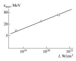
**Fig. 2.** Maximum proton energy vs. the laser intensity. The square, circle, and triangle mark the results of [8, 9, 20], respectively. The solid line is the fit  $\epsilon_{\text{max}} \simeq 3.6 \sqrt{I/10^{18}}$  MeV, where I is in W/cm<sup>2</sup>.
