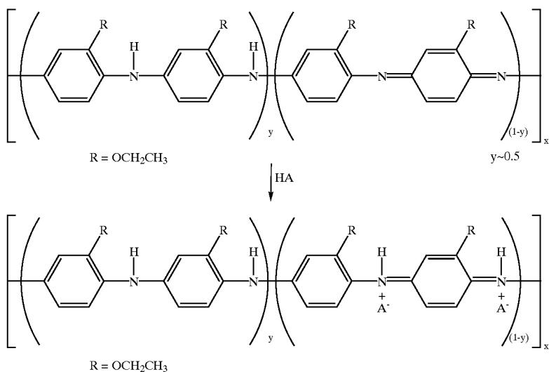
The ethoxy substituted polyaniline in the non-doped form (base) can be readily dissolved to a 10% by weight solution in NMP, and spun at various rpms to form films of different thicknesses (184,339 and 477 nm, respectively). Films from this polymer are very homogenous and well adherent. Even the thinnest film behaves as a perfect barrier to oxygen, as 25
