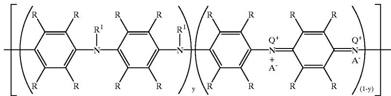
The emeraldine salt is the highly conducting form. The conductivity of the polyaniline can range from  $10^{-10}$  ohm $^{-1}$
