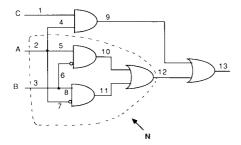
Fig. 7. A testable realization for  $A \oplus B$ .
