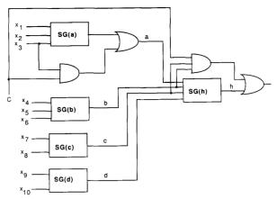
Fig. 6. Parity-testable design for the overall circuit.
