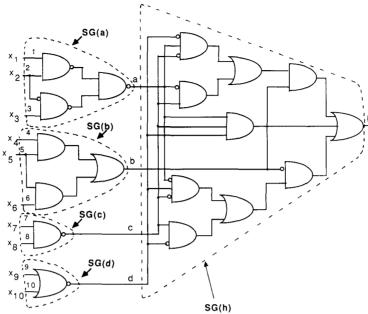
Fig. 2. An illustrative circuit for parity testing.
