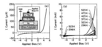
FIG. 2. (a) The I–V curve of a Ni-B<sub>5</sub>C $_{1+\delta}/B_5$ C diode at 296 K with a "low" Ni concentration, and (b) the temperature dependence of the rectifying behavior of this diode. The inset in (a) is a schematic of the diode construction.
