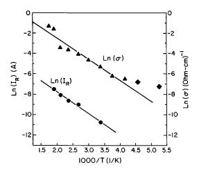
FIG. 3. (a) The natural log of the conductivity of Ni-B<sub>5</sub>C<sub>1+ $\delta$ </sub> as a function of reciprocal temperature, where the line is a fit of the data, and (b) the natural log of the leakage current of a Ni-B<sub>5</sub>C<sub>1+ $\delta$ </sub>/B<sub>5</sub>C diode as a function of reciprocal temperature.
