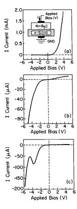
FIG. 1. The diode I–V characteristics of (a) B<sub>5</sub>C/n-Si(111), (b) Ni-B<sub>5</sub>C<sub>1+ $\delta$ </sub>/n-Si(111) with "low" nickel concentration, and (c) the I–V curve of a tunnel diode of Ni-B<sub>5</sub>C<sub>1+ $\delta$ </sub>/n-Si(111) with "high" nickel concentration. The inset in (a) is a schematic of the Ni-B<sub>5</sub>C<sub>1+ $\delta$ </sub>/n-Si(111) diode.
