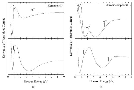
**Figure 4.** (a) A comparison of electron transmission spectra for camphor reported in [2] (lower panel) and [7] (upper panel). Vertical lines indicate resonance energies. (b) A comparison of electron transmission spectra for 3-bromocamphor obtained in this work (upper panel) and reported in [2] (lower panel). Vertical lines indicate resonance energies.
