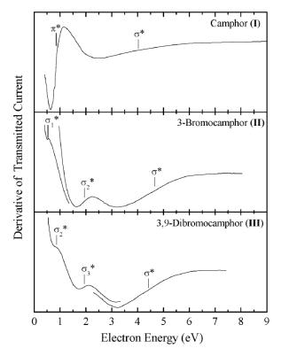
**Figure 3.** Derivative with respect to electron energy of the current transmitted through gas phase camphor, 3-bromocamphor and 3,9-dibromocamphor. Vertical attachment energies (VAEs) are indicated by short vertical bars and labelled to indicate the orbital responsible for the resonance.
