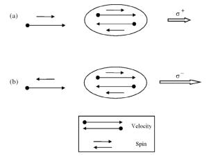
**Figure 2.** Schematic diagram of polarized electron scattering by a target of a given chirality (see the text). The arrows of different sizes to the right indicate different forward-scattering cross sections for spin-forward (right-handed; +) electrons versus spin-backward (left-handed; -) electrons.
