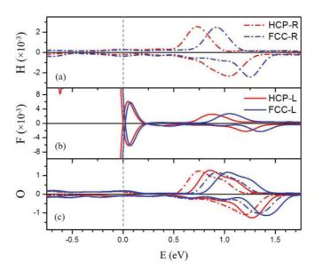
FIG. 4. (Color online) Comparison of the density of states (DOS) at the interface of the Co/PVDF/O/Co MFTJ for the hcp- and fcc-adsorption sites. Induced DOS on (a) H and (b) F atoms at the oxidized interface; and (c) DOS on the O atom at the interface. Red/dark gray (blue/medium gray) lines show results for O in hcp (fcc) sites. Solid (dashed-dotted) lines indicate polarization pointing left (right). Induced DOS on H and F atoms is multiplied by  $10^3$ .
