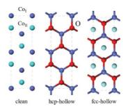
FIG. 2. (Color online) Atomic structure of clean and oxidized Co surface. O atoms (red/dark gray) are in either the hcp- or fcc-hollow sites. Blue (medium gray) Co atoms ( $Co_I$ ) are at the surface and light blue (light gray) Co atoms ( $Co_{II}$ ) are at the layer immediately below the surface.
