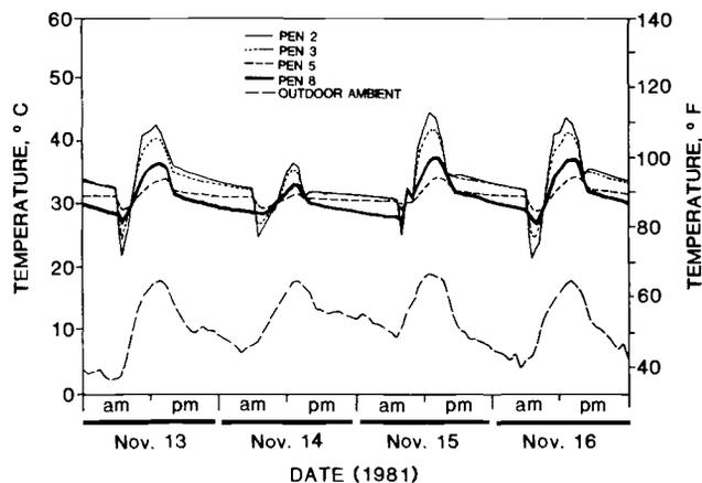
Fig. 10—Air passageway temperatures along the in-floor heat distribution-storage system with manual operation of collector fan.
