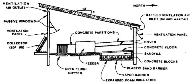
Fig. 3—Schematic of the solar MOF nursery cross-section.
