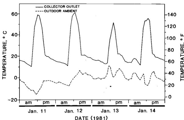
Fig. 6—Air temperatures at the outlet end of the active solar collector on sunny days (Paus).
