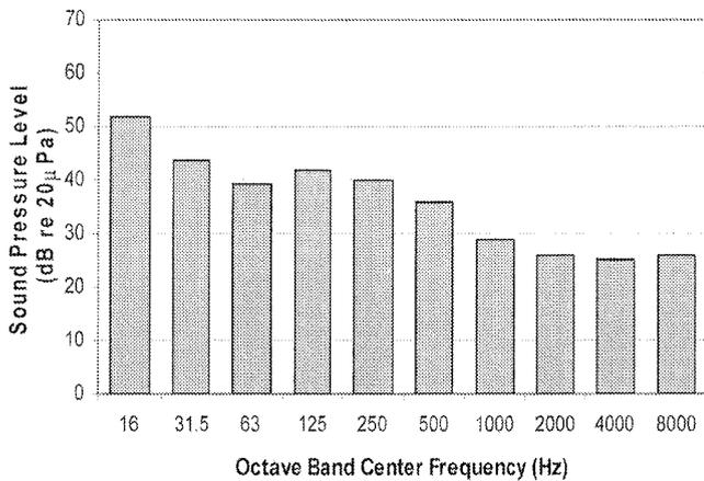
**Figure 2** Frequency character of test chamber background noise levels.
