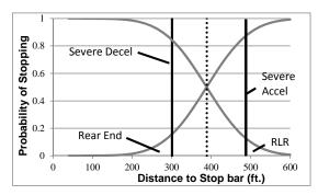
Fig. 1 - Critical distances along probability of stopping curve
