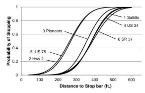
Fig. 3 - Critical distances along probability of stopping curve
