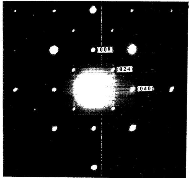
FIG. 4. Selected area diffraction pattern of the  $\alpha\text{-Zn}_3\text{As}_2$ . The satellite spots near the (008), (040), and (024) reflections arise from the ordering of the vacancies on the Zn sublattice.
