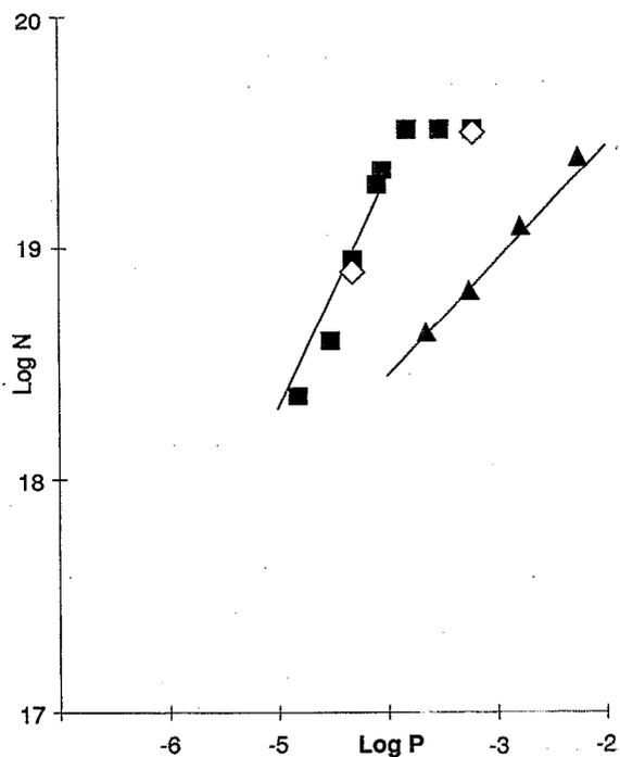
FIG. 3. Zn concentration ( $\text{cm}^{-3}$ ) vs  $P_{\text{Zn}}$  (atm) for growth, as measured by CV ( $\blacksquare$ ) and SIMS ( $\diamond$ ), and for diffusion ( $\blacktriangle$ ). The surface concentration, taken from the diffusion studies, follows the expected dependence on  $P_{\text{Zn}}$  when solid-vapor equilibrium can be approximated.
