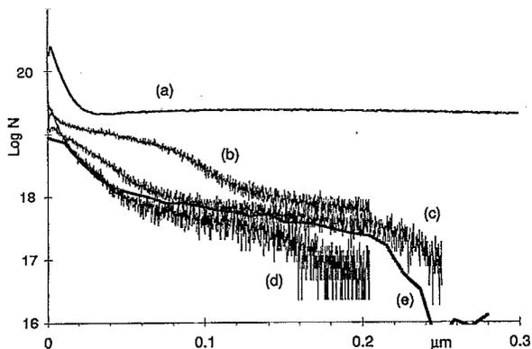
FIG. 2. Zn concentration ( $\text{cm}^{-3}$ ) vs depth ( $\mu\text{m}$ ) below surface after a 2 h diffusion with  $P_{\text{Zn}}$ =(a)  $5.67 \times 10^{-3}$  atm, (b)  $1.70 \times 10^{-3}$  atm, (c)  $5.67 \times 10^{-4}$  atm, and (d)  $2.27 \times 10^{-4}$  atm. Curve (e) shows the Zn concentration profile below a Zn-doped epilayer after a 2 h growth period.
