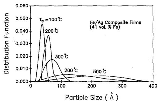
FIG. 3. Particle-size distributions of Fe/Ag composite films (41 vol % of Fe) at substrate temperatures of 100, 200, 300, 400 and 500 °C.
