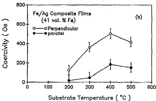
FIG. 5. Magnetic coercivities at 25 °C of Fe/Ag composite films containing (a) 27 vol % of Fe and (b) 41 vol % of Fe deposited at various substrate temperatures. (Data measured when the applied field was both perpendicular and parallel to the film surface are shown.)
