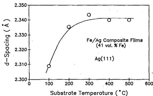
FIG. 2.  $d$  spacing of Ag(111) vs the substrate temperatures
