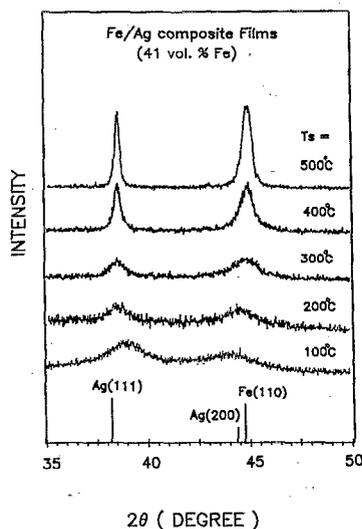
FIG. 1. X-ray  $\theta$ - $2\theta$  scans of Fe/Ag composite films prepared at substrate temperatures of (a) 100 °C, (b) 200 °C, (c) 300 °C, (d) 400 °C, and (e) 500 °C. The Miller indices for elemental Fe and Ag are shown on the bottom of the figure.
