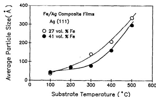
FIG. 4. Average particle size in Fe/Ag composite films (27 and 41 vol % of Fe) vs substrate temperature.
