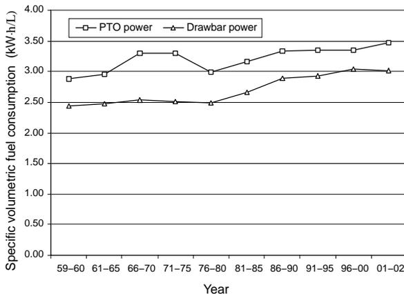
**Figure 1. Trends in specific volumetric fuel consumption.**
