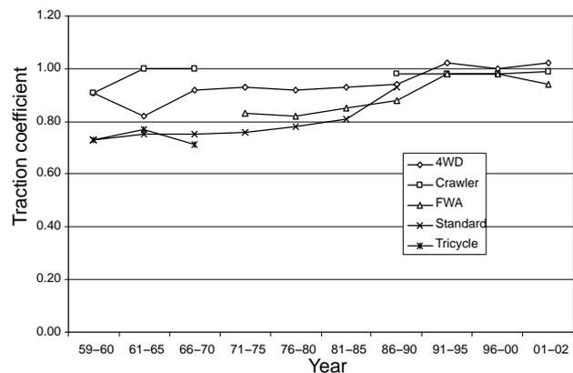
Figure 13. Average traction coefficient by chassis type.
