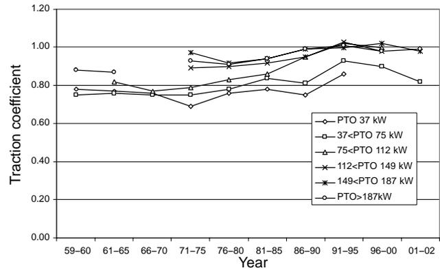
Figure 12. Average traction coefficient by PTO power level.
