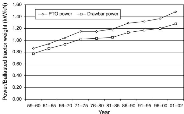
Figure 6. Changes in power produced per unit weight of ballasted tractor.
