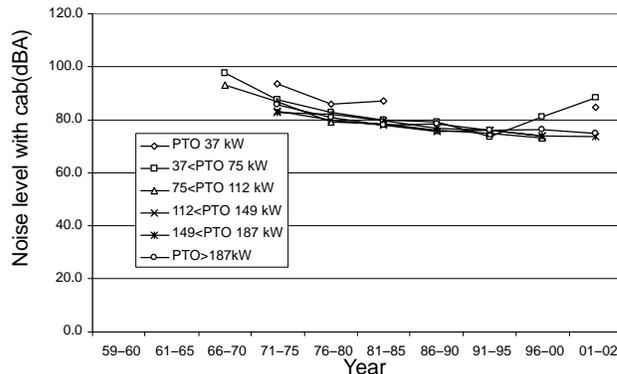
Figure 15. Maximum sound level within the cab.
