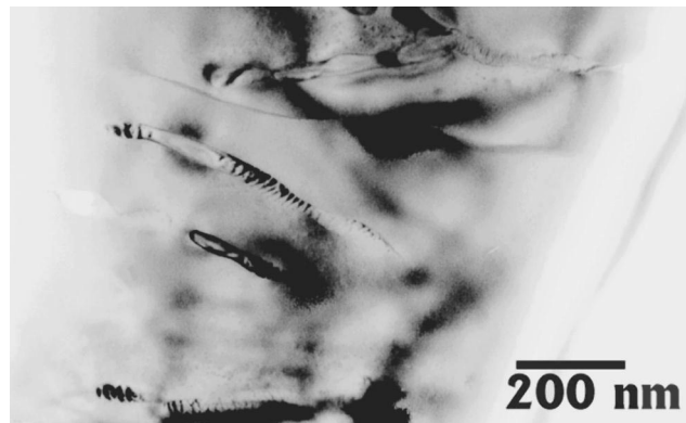
FIG. 3. TEM micrograph of the top layer of the 10 m/s ribbon showing very large 2-14-1 grains with aligned filaments of Fe.
