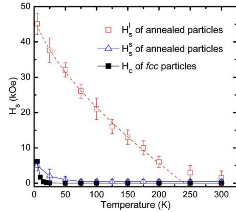
FIG. 5. (Color online) Temperature dependence of switching field  $H_s^1$  and  $H_s^2$  of the annealed 3 nm nanoparticles and the coercivity of the as-synthesized particles. The dashed line is the Kneller-Sharrock fitting of the  $H_s^1$  data.
