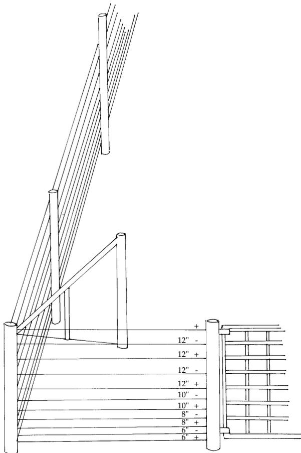
Fig. 8. A high-tensile electric fence can exclude elk.
