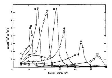
Figure 2. Doubly-differential cross sections in energy for 0° emission of electrons in H\*+He collisions at proton energies between 20 keV and 100 keV [33]. An apparent midvelocity secondary maximum, evident between 40 and 60 keV, disappears at higher energies, and, if present, is not resolved at lower ones. See also refs. 7,8, and 18.
