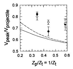
**Figure 3.** Position of peak in velocity space for  $10^{\circ}$  emission in 50 keV (open circles) and 100 keV (solid circles) proton impact ionization. Left two data points are for Ne targets, the middle two are for Ar, and the righthand two are for He.  $Z_p=1$ ;  $Z_p$
