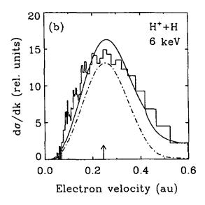
Figure 1. Relative electron yield vs. electron velocity for 6 keV H\*+H collisions. Projectile velocity divided by two is indicated by the arrow. The dash-dot curve indicates the theoretical prediction for the saddle-point electron contribution; the solid curve is the total yield prediction, fitted with one height parameter to the experimental results. Data and theory of ref. [20].
