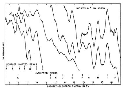
Fig. 2. Energy spectrum of electrons from 100-keV Ar<sup>+</sup>-Ar collisions. Resolution about 0.2 eV.
