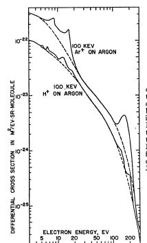
Fig. 1. Doublydifferential cross-sections for ejection of electrons from argon by protons and argon ions at 100 keV. Electrons are detected at 160° from the beam direction. Resolution from 0.5 eV at 3 eV energy to 12 eV at 300 eV.
