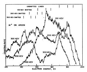
Fig. 3. Energy spectrum of electrons from Ar<sup>+</sup>-Ar collisions. Resolution about 3 eV.
