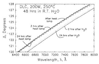
FIG. 5. Ellipsometric delta parameter vs wavelength at various times after removing the sample from water, as listed. Sample deposited at 200 W, 250 °C, soaked in room temperature water for 48 h. After removing from water, it was kept in a room atmosphere.
