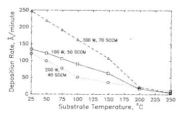
FIG. 1. Deposition rate vs substrate temperature for three different power level/flow-rate settings.
