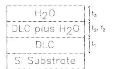
FIG. 2. Structure model assumed for analysis of DLC moisture studies.
