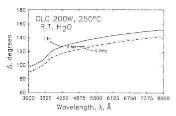
FIG. 7. Ellipsometric delta parameter, same conditions as in Fig. 6.
