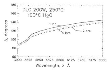
FIG. 9. Ellipsometric delta parameter vs wavelength for samples soaked in 100  $^{\circ}$ C water for 1–4 h.
