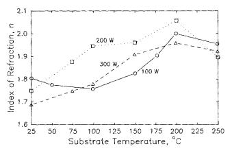
FIG. 3. Optical index of refraction vs substrate temperature for three different power levels.
