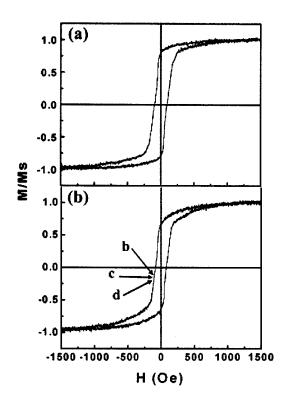
FIG. 2. Hysteresis loops of Co–C nanodot arrays with the field applied (a) along the easy axis direction and (b) along the direction  $30^{\circ}$  off easy axis. Points (b), (c), and (d) in (b) correspond to the fields in Figs. 3(b)-3(d), respectively.
