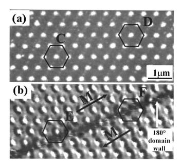
FIG. 4. (a) Topographic image and (b) MFM image of a 180° domain wall in Co–C nanodot arrays. The domain wall is located in the matrix, shown in hexagon E, and on the dot, shown in F. Hexagons C and D are corresponding hexagons in the AFM image.
