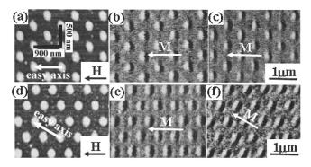
FIG. 1. AFM and MFM images of Co–C nanodot arrays. The top three images were measured with field applied along the easy axis direction. (a) AFM image, (b) MFM image in the saturated state under a 425 Oe field, (c) MFM image in the remanent state. The bottom three images were measured with field applied along the direction 30° off easy axis. (d) AFM image, (e) MFM image in the saturated state under a 425 Oe field, (f) MFM image in the remanent state.
