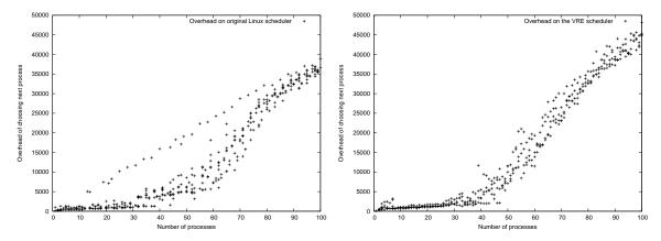
Figure 5: The overhead is a linear function of the number of processes under bother the original Linux scheduler and our scheduler. The overhead of our scheduler is a little bit higher than the original Linux scheduler.
