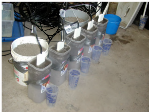
Figure 2. Performing soil TDR experiments in the laboratory.
