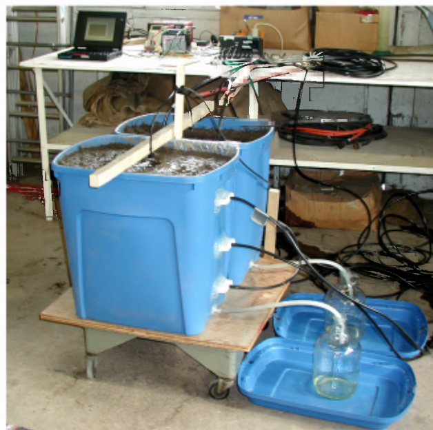
Figure 3. Laboratory lysimeter setup.
