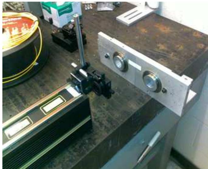
**Figure 2.2:** Schematic of the  $\pi$ FBG fabrication setup (left), reflection spectrum of the original regular FBG and during the CO<sub>2</sub> laser heating process (right), and image of the physical setup (Bottom).
